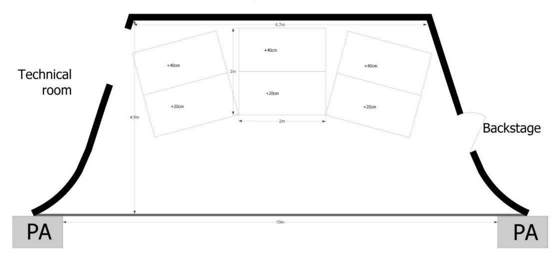
Temporary stage elements (20pcs) can be used as stage extension or as risers in different combinations.
